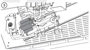
Replace with the correct size plate and secure the 2 nuts. Ensure that the lower edge of the plate is located over the venturi flange.
