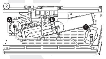
Holding the injector with a spanner:
