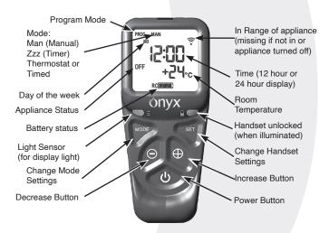
The Icon at the bottom of the screen displays the battery condition of both the batteries in the handset and in the appliance alternatively.
