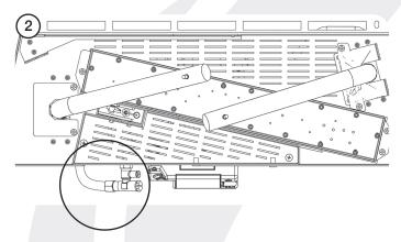
**PURGE THE SUPPLY PIPE**. This is essential to expel any debris that may block the gas controls.
